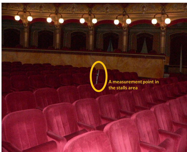
Fig. 5 Acoustic measurements in the stalls area, with the indication (in yellow ) of the measuring microphone at a seat
