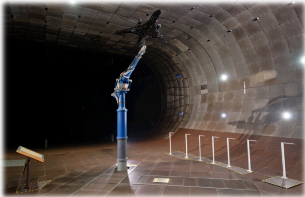
Figure 8. A photograph of AMELIA mounted in the 40ft by 80ft test section at the NFAC at Ames Research Center at the highest angle of attack tested (+25°).
