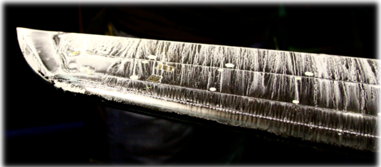
Figure 26. A photograph of the AMELIA wing tip with the oil flow visualization technique illustrating the wing tip flow physics does not follow the inboard section of the wing where the momentum flow has attached the flow exiting the plenums.
