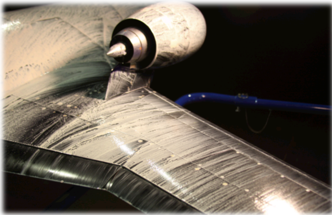
Figure 25. A photograph of AMELIA utilizing oil flow visualization to verify the quality of the flow exiting the circulation control wing plenums at 40kts and a momentum coefficient of 0.8.
