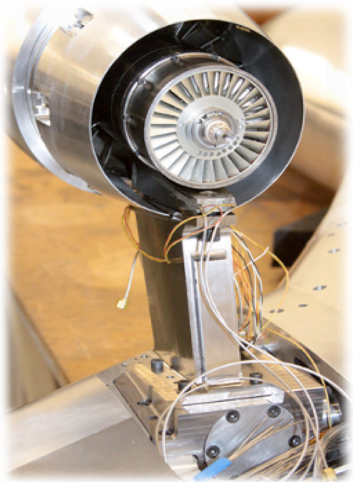
Figure 6. A photograph of the Model 441 TPS unit installed in the nacelle mounted on AMELIA.
