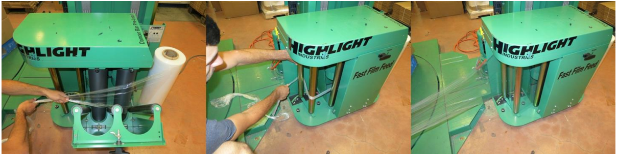
Figure 33: Feeding the Film between Rollers [7]
