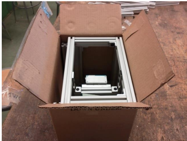
Figure 9: Extruded Aluminum Fixture in RSC
