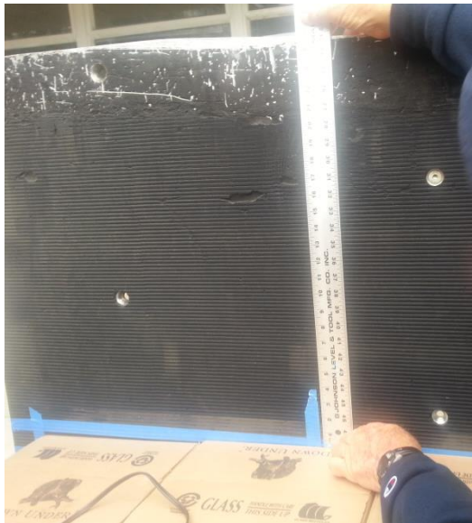
Figure 38: Measuring Load Position between Clamp Pads
