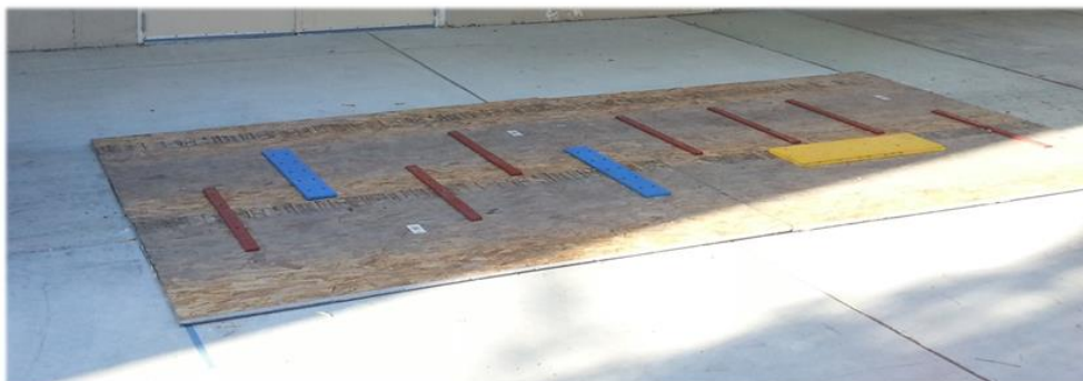
Figure 12: Plate Obstacle Course ISTA 3B-2013
