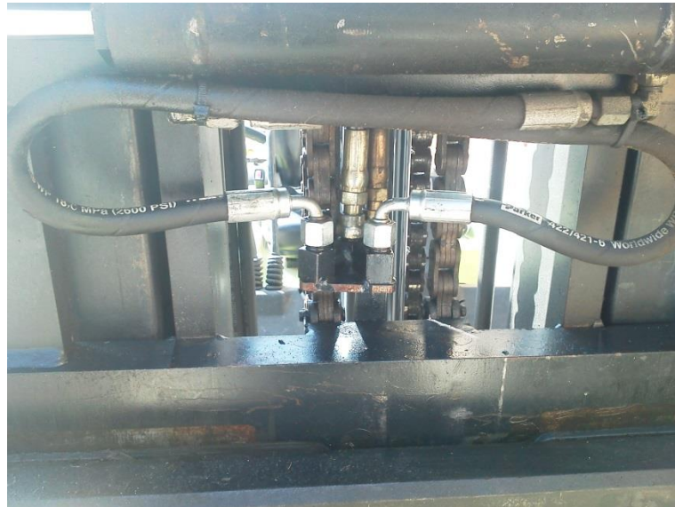
Figure 26: Side Shift Fittings
