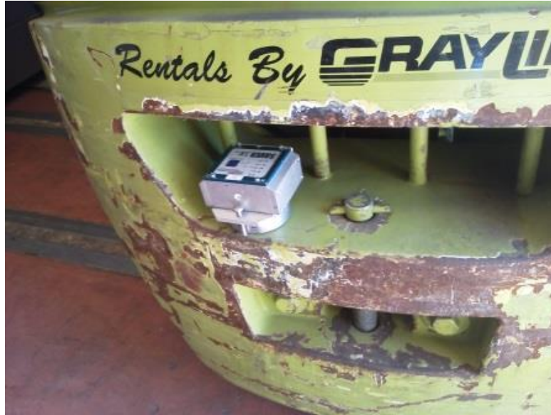
Figure 10: Data Recorder Position Truck
