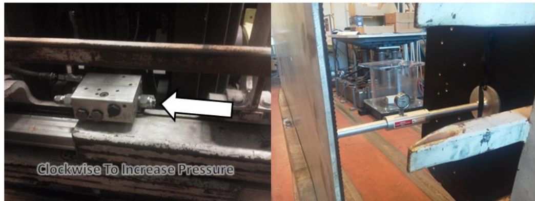
Figure 29: Adjusting Maximum Clamp Force Pressure
