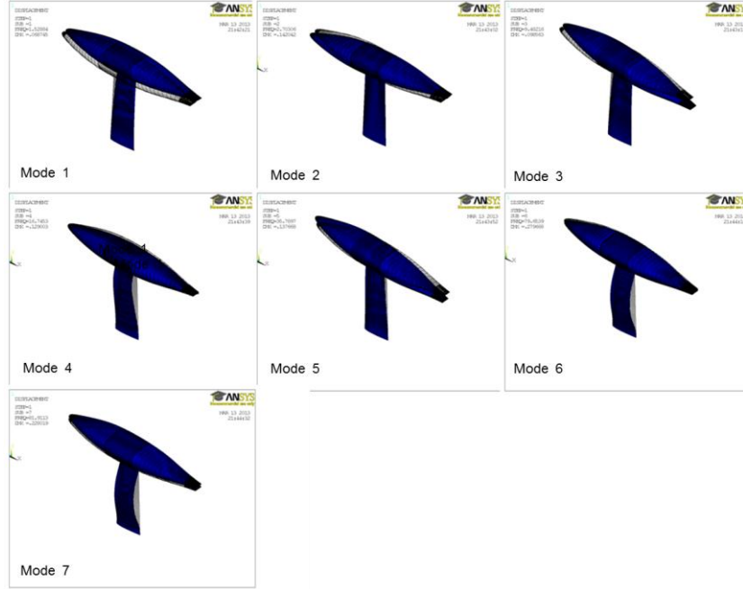
Figure 6 Mode Shapes of the keel bulb
