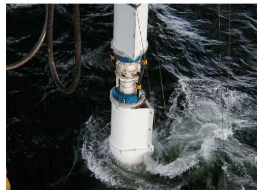
Figure 1 A Typical Installed Riser Fairing.
