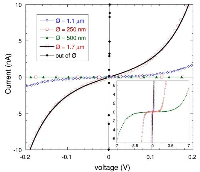
FIG. 3. (Color online) Zoom of the  $I/V$  curves measured inside (circles) and outside of the patterned areas for an as-grown LCMO film with a capping layer of 30 nm of Pt. The lines through the experimental points correspond to fits using the Simmons model. Inset:  $I/V$  curves in the extended range.
