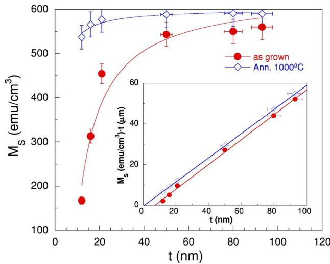
FIG. 1. (Color online) Saturation magnetization ( $M_s$ ) of LCMO films as a function of the thickness ( $t$ ). Inset: Fit of  $M_s t$  product to estimate the nonmagnetic layer.
