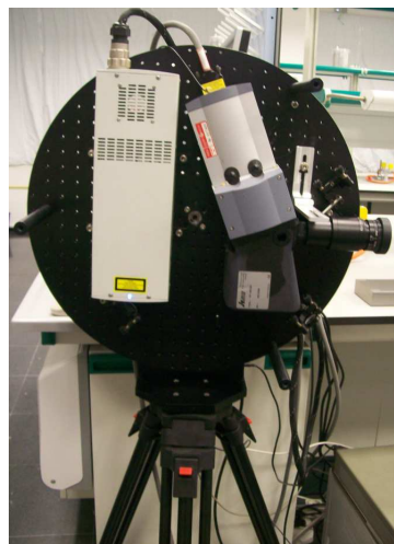
Figure 1: Actual set up of LidArt: laser (left), ICCD (top right) and imaging spectrograph (bottom right) are mounted on a circular optical table
