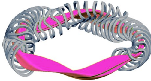
Figure 1.7: A cartoon showing the coil and plasma configuration in a stellarator[EFDA, 2013a].
