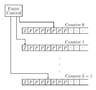
Figure 3: A k-counter machine (CM(k)).
