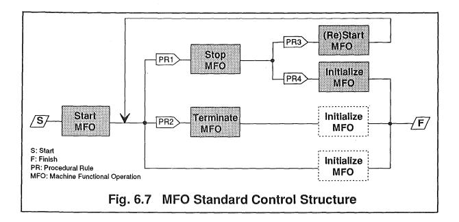
The action in the dotted blank box indicates that the service is not issued by the Activity Control. Internally, it is automatically triggered by the Machine Front-End. For example, after a *Start MFO Service Request* issued by the Activity Control has been sucessfully executed, the Machine Front-End should itself execute the Initialize service block of the Control Model, not because of an *Initialize MFO Service Request* issued by the Activity Control.
