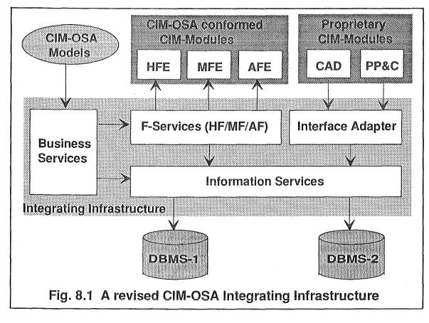
Keys are: HFE: Human Functional Entity, AFE: Application Functional Entity, PP&C: Production Planning & Control, HF: Human Front-End, AF: Application Front-End, MFE: Machine Functional Entity, CAD: Computer Aided Design, F-Services: Front-End Services, MF: Machine Front-End, DBMS: Data Base Mgmt. System.
