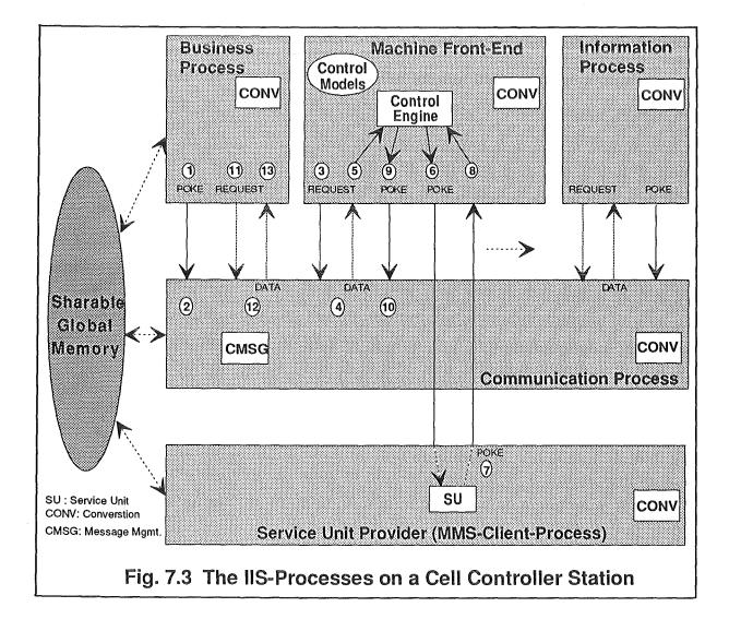
The prototype uses the concept of sharable global memory to store the messages to be transferred between the processes. Each message unit has a unique identifier assigned to it. For the message passing, the method of *message identifier transfer* is
