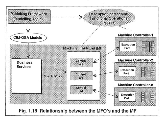
Furthermore, the Machine Front-End has a two-fold nature in the IIS environment of the client-server model: it acts as a client and as a server. The following chapters will describe the problem statement and the proposed solution in detail.
