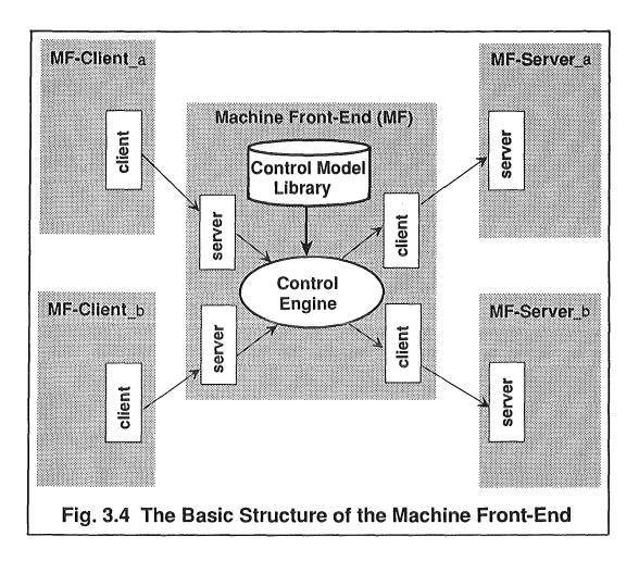
The *Control Model Libray* actually represents a database containing control models (all the MFO-specific control knowledge of an application) to be interpreted by the Control Engine. It participates in the transformation of the *MF-Service Indications* (*MFO calls*) into a sequence of service requests to be sent to its MF-Servers.
