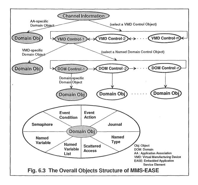
In MMS-EASE, a *VMD Control Object* (VMD Control) is used to represent a VMD. It is linked with its preceeding and succeeding *VMD Control Objects*. This means that several VMD's can be established for a server application. This object contains the VMD-specific information: a VMD-specific Domain Object, pointers to the Domain, Program Invocation, Operator Station and Named Domain Control object, etc.
