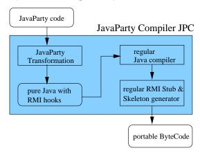
In the following sections we present the central ideas used for the transformation of JavaParty into Java plus RMI hooks. Many details of the transformation (e.g., object equality, this, synchronization, etc.) must be omitted.
