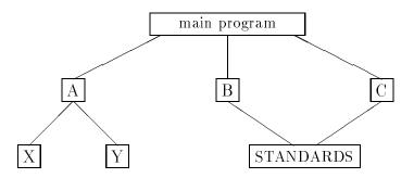
All global objects of the modules A, B, and C are visible in the main program unit, but there is no access to the global objects of X, Y and STANDARDS from the main program.
