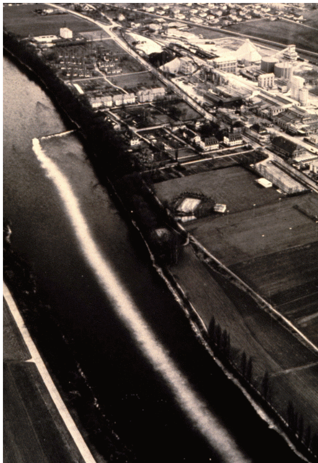
Fig. 3: Aerial photograph (ca. 1960) of an industrial discharge located near the middle of the regulated River Rhine upstream of Lake Constance (Bodensee). The gradual lateral plume growth of the pollutant is typical for mixing processes in rivers. (Photograph courtesy of D. Vischer, Zurich)
