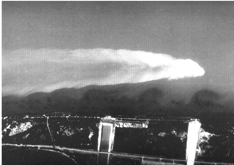
Fig. 5: Surface plume in a long shore coastal current produced by a submerged sea outfall. The infrared image shows the plume produced by the cooling water discharge from a power plant at the western coast of Florida.
