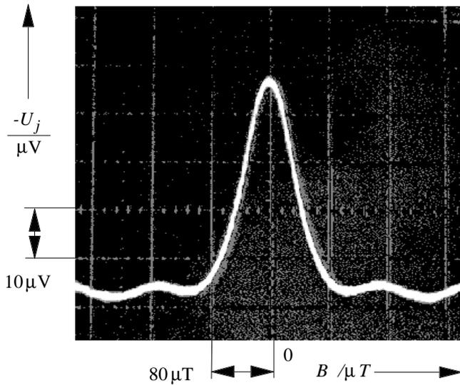
**Fig 2:** Voltage versus magnetic induction at 77 K of a 6  $\mu\text{m}$  wide step edge junction according to Fig. 1 at constant current  $I_G$ .
