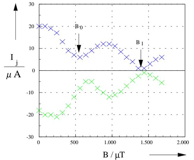
**Fig. 3:** The Josephson current  $I_j$  of a step edge junction at 77 K versus magnetic induction  $\mathbf{B}$ .
