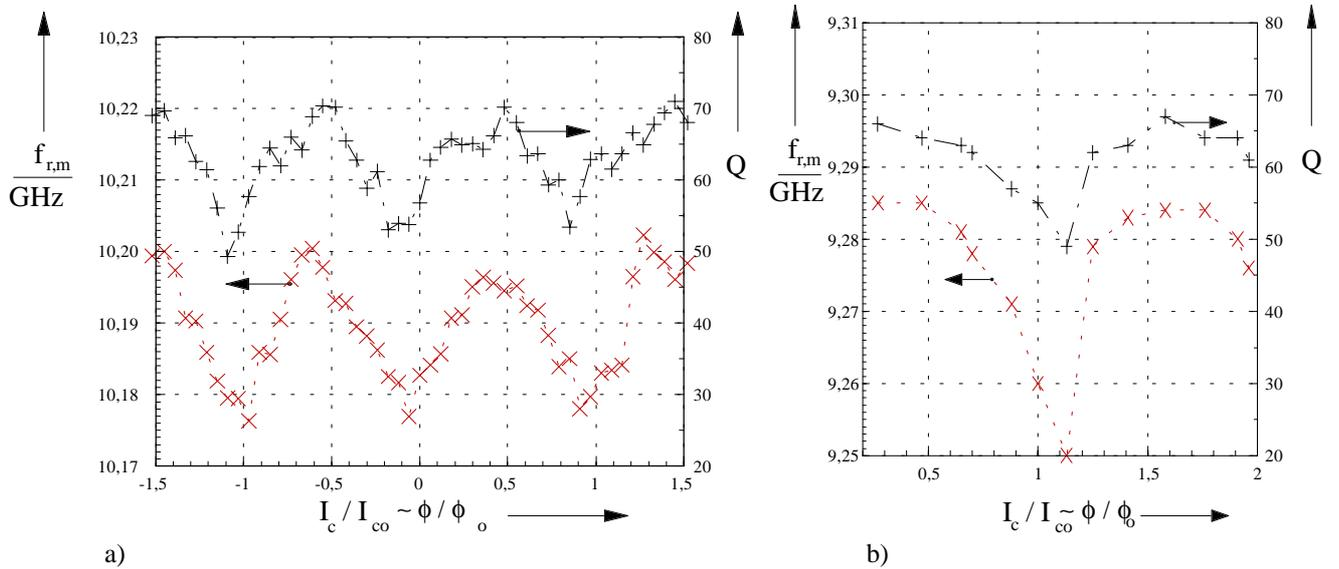
**Fig. 5:** a) Measurement results: Resonance frequency  $f_{r,m}$  and quality factor  $Q$  versus the normalized control current. The center frequency  $f_{r,m} = (f_1 + f_2)/2$  is calculated from the measured 3 dB - frequencies  $f_1, f_2$ . b) Simulated results with  $I_o R_n = 135 \mu\text{V}$  [7].
