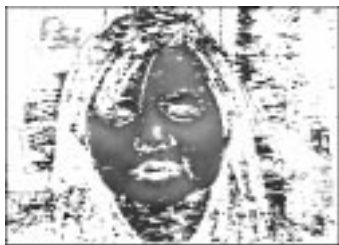
Figure 1. Example of the output of the Face Color Classifier. Dark areas are classified as skin-colored.
