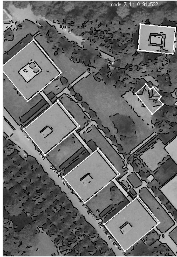
Figure 6: Result of the model based verification. Dark lines: image primitives; white lines: solution.
