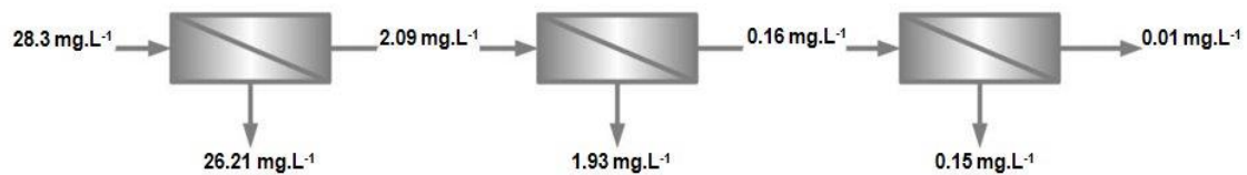
Figure 39. Methane outlet concentrations for PDMS modules in series assuming c. 93% removal efficiency for every contactor; V_L of 0.00036 \text{ m.s}^{-1} .
