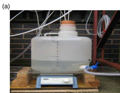
Figure 19. Equipment used for water saturation with methane and/or carbon dioxide: (a) water saturator; (b) sparging head.
