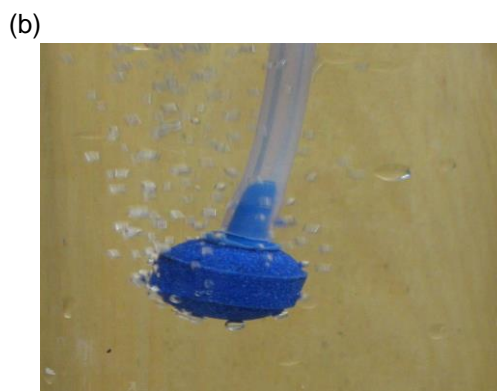
Figure 19. Equipment used for water saturation with methane and/or carbon dioxide: (a) water saturator; (b) sparging head.
