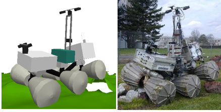
Fig. 9. A predicted placement of Lama on a DEM (left) and the corresponding placement on the real terrain (right)
