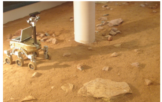
Fig. 7. Rock traversal experiment setup: rover is shown at its starting position. It must traverse over a “rock field” to reach a goal region to the right (out of the picture).
