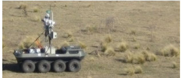
Fig. 1: Multiple grass tussocks in front of the vehicle that are usually seen as obstacles by the LIDAR.
