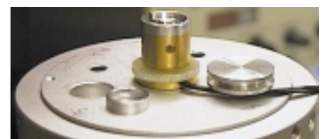
Fig. 5: The modified TE detector mounted on the sample stage like a specimen stub; the AI TEM-grid holder is placed on top of the TE detector housing, the annular aluminium shield is on the left
