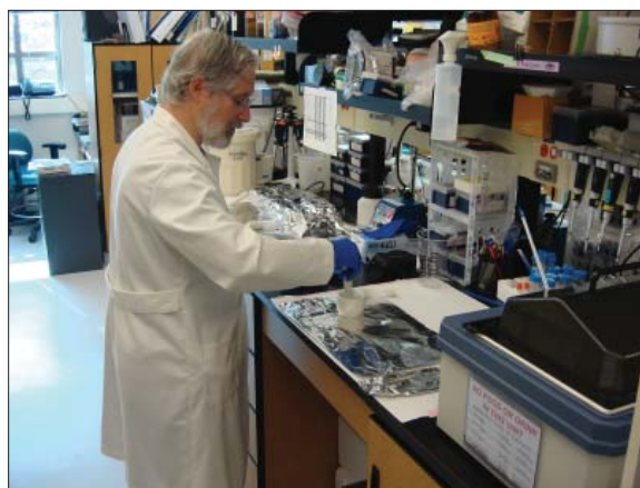
Grinding of coral tissues in preparation for analysis of chemical contaminants.
