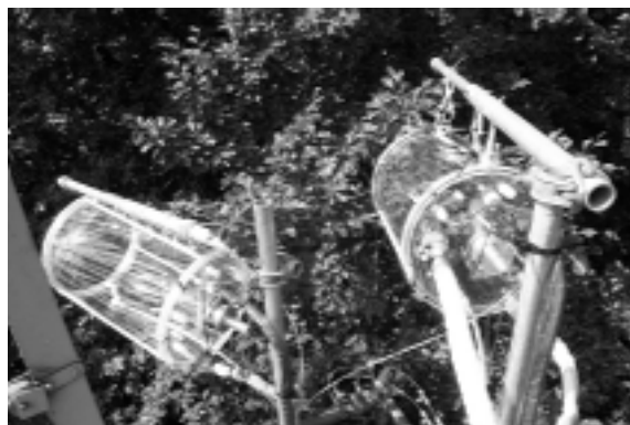
Figure 1. Two enclosures (stabilised Teflon film bags), one is an empty reference, and the other one is enclosing a branch to investigate trace gas exchange between plants and the atmosphere acting like a stethoscope to listen. Emission measurements are accompanied by the determination of CO 2 -exchange (photosynthetic assimilation, respiration) and water transpiration (Figure 2). Flushing air is mostly ambient but is cleaned from oxidants for the detection of reactive compound emissions.
