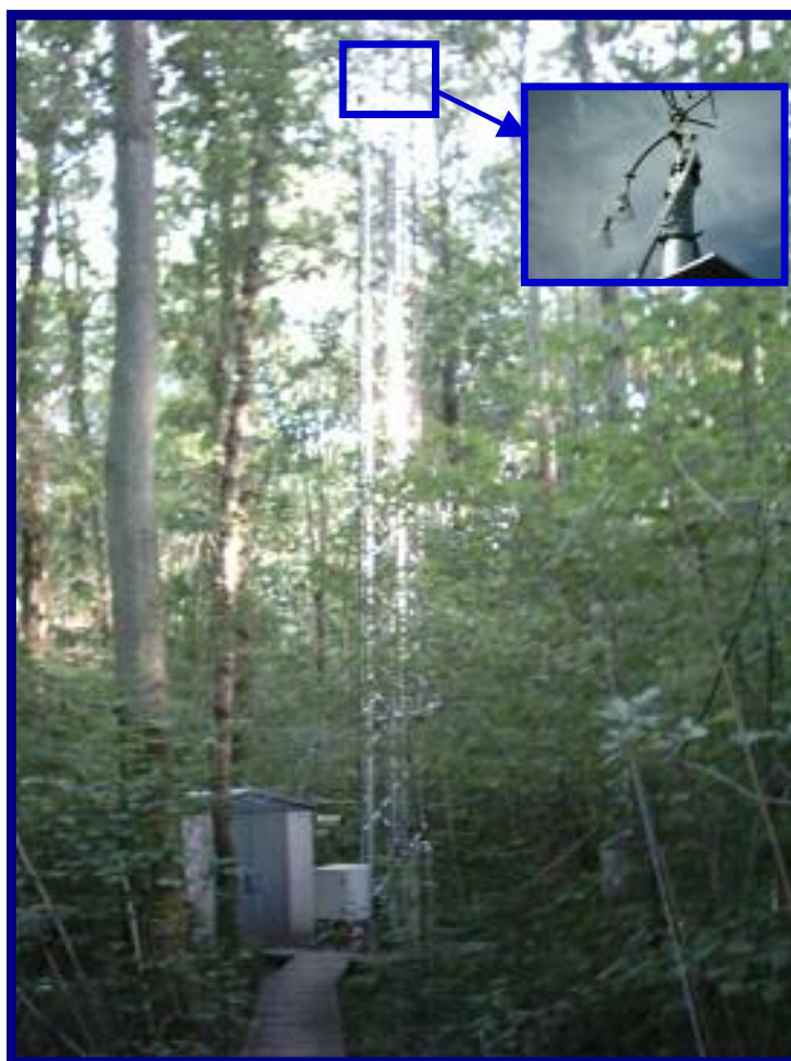
Figure 1. Measurement site in Alice Holt forest, showing the access tower and (inset) the PTR-MS inlet immediately below the sonic anemometer.
