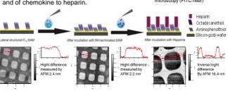
• Procedure: A PDMS stamp with a lateral pattern was loaded with a solution of octadecanethiol. The thiol pattern was printed on a gold coated silicon wafer. The silicon wafer was incubated with aminophenolthiol and then with heparin for 1 hour. Hight profiles of the surface were measured after every incubation step to control surface topography.
