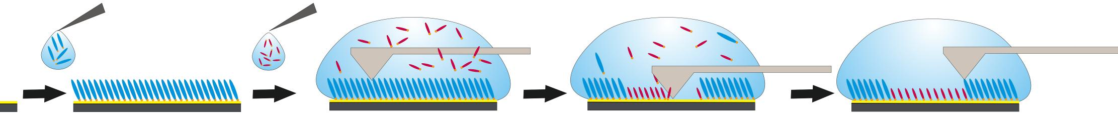
The matrix SAM is covered with an ethanolic solution of another SAM. After the removal of the matrix SAM molecules from the gold surface by the AFM tip, the vacant sites are filled up immediately with molecules out of the ethanolic solution and can be ivestigated by AFM with the same AFM-tip.
