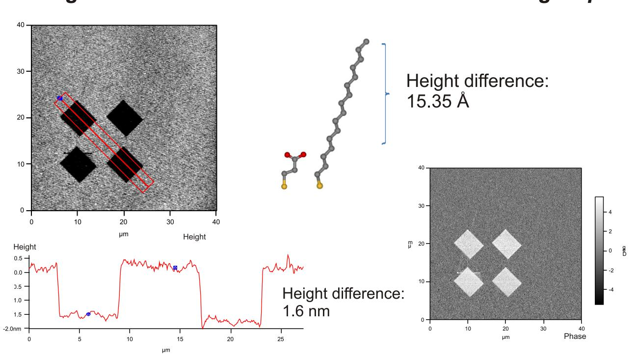
Nanografting area of mercaptopropionicacid (MPA) in decanethiol with the corresponding cross section and the phase image.
