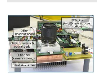
KIT High Speed Streaming Camera Resolution: 2048 x 1088 @ 10 bits:
