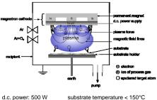
d.c. power: 500 W substrate temperature < 150°C
