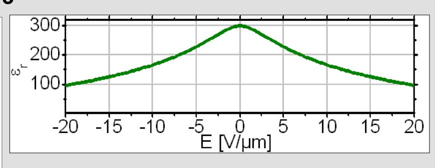
BST shows a nonlinear dependence of the permittivity on a static electrical field strength
