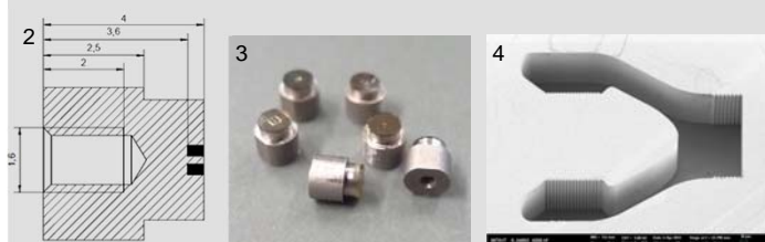
Figure 2: 1) structured nickel, 2) dimensions of the mold inserts, 3) LIGA mold inserts, 4) SEM figure of a LIGA cavity
