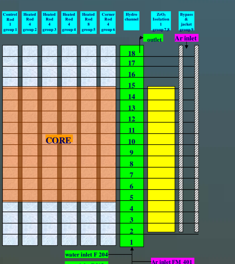
Fig. 3. SOCRAT nodalization for QUENCH-16
