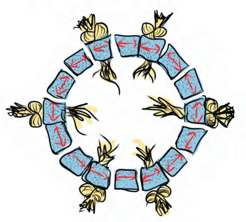
Wood rays in trees interlock growth stress compressed external sapwood with internal wood loaded in circumferential tension.
