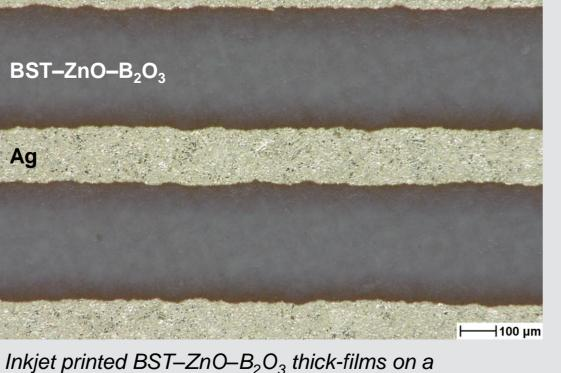
screen printed Ag thick-film, sintered at 850°C Multilayer capacitor with evaporated Au top-electrode: → Tunability:  $\tau = 30\%$  (@ 40 V, 3 GHz)  $\checkmark$
