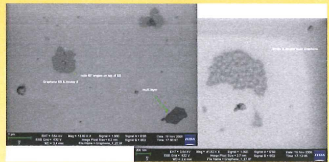
Fig. 4 SEM of graphene single sheet, double sheet and multilayer. Contrast is due to the presence or absence of delocalised \pi -bonding. The thickness of the monolayer graphene is 2.42Å (SEM performed by Dr. Heiner Jaksch, Carl Zeiss NTS GmbH, Oberkochen, Germany)
