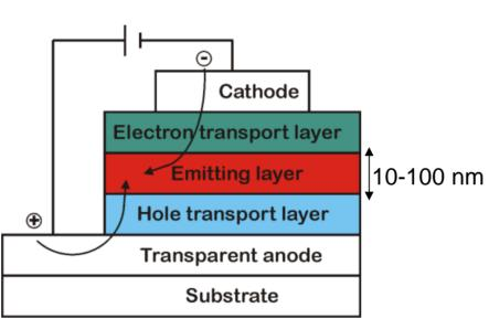
OLED structures, the possibility to characterise the material mixing between layers during coating and drying, and the comparison to evaporated layers is crucial.
