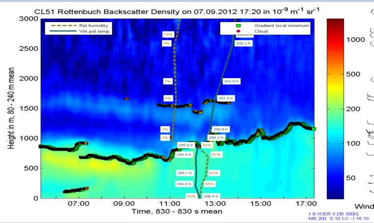
Development of mixed layer height, at the TERENO-Ammer site Rottenbuch, determined from measurements by one of four ceilometers (VAISALA CL51) in the observatory, using the minimum gradient nethod
