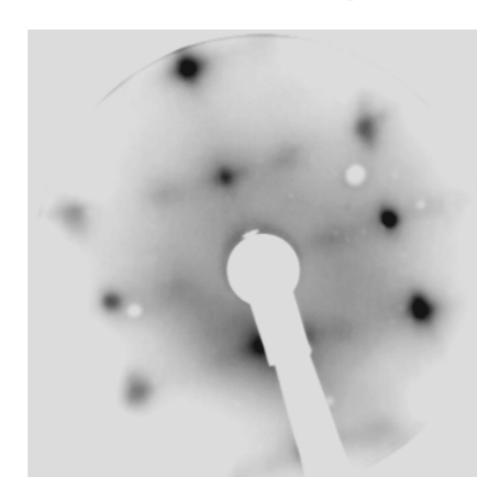
LEED: (2x1) – Phase of CO 2 on ZnO (10 \bar{1}0 )
