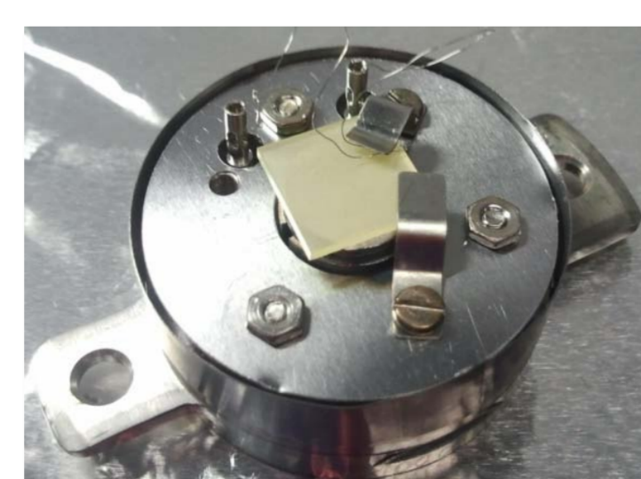
ZnO (10 \bar{1}0 ) single crystal on sample holder.
