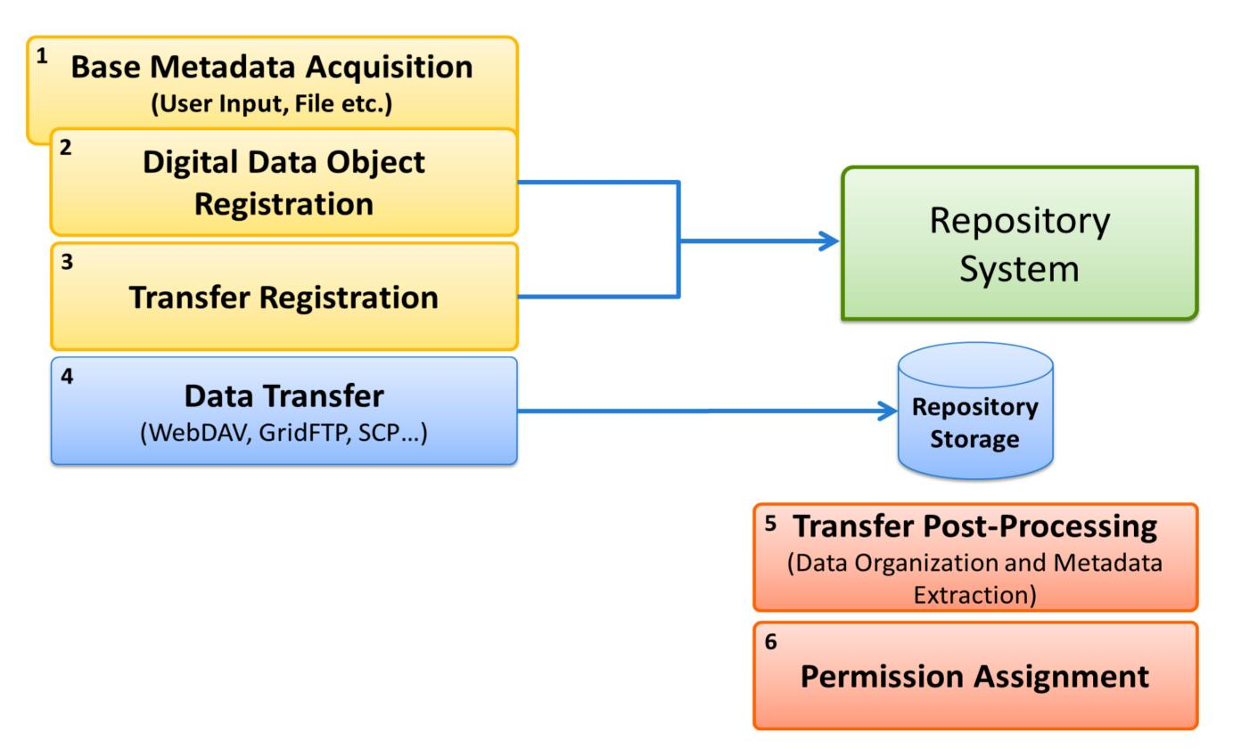
Data ingest workflow including digital object registration (1,2,3), data transfer (4) and post-ingest operations (5,6).
