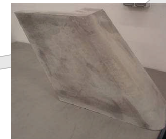
Step C: HIPped body of the double wall structure
