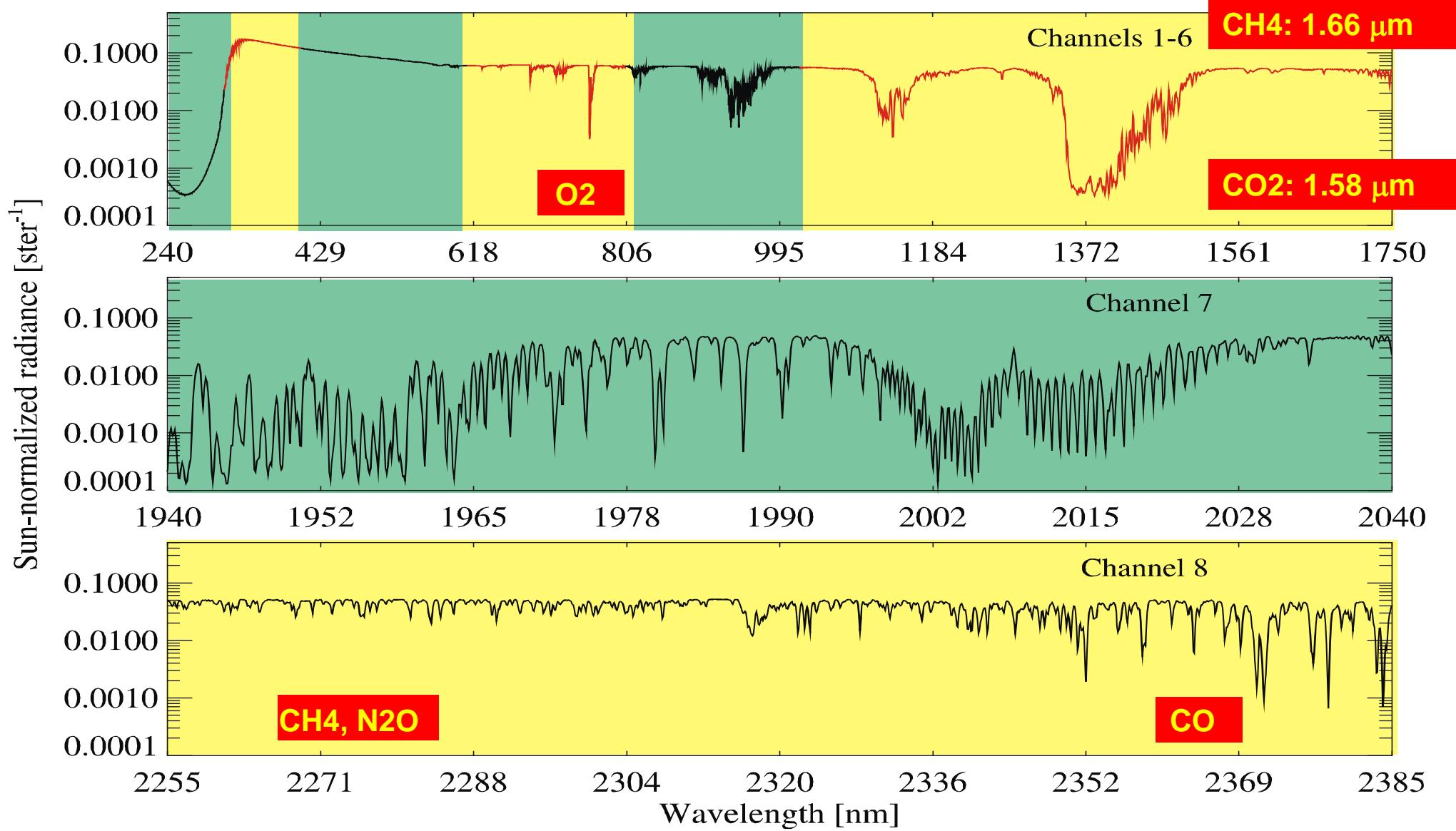
After validation in 2005, the SCIAMACHY icing issue was overcome by re-implementing SCIA retrievals from channel 8 to channel 6.
