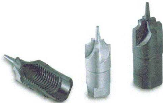
Hard metal WCxCo with different Co-contents (16% and 6%), ARBURG
