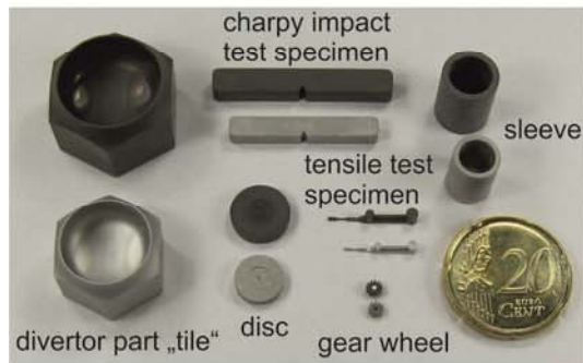
Green parts (dark) Finished parts (bright)
