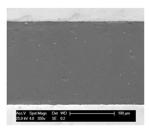
SEM: Good adhesion of Ti and W surfaces!
