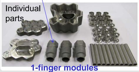
9-finger module (W) for HHF tests (Efremov, <u>HELOKA</u>) 9-finger module (brass) for NDE (<u>SATIR</u>, CEA)
