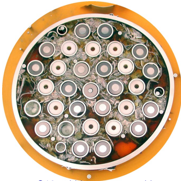
Q12: rubble on spacer grid consists of spalled cladding scales and fragments of partially oxidized cladding
