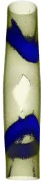
hydrogen bands inside cladding detected with n^0 - radiography: max 2500 wppm hydrogen content
