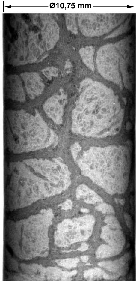
Crack development in the cladding, cooled down with steam. Crack density ~ 4 cm/cm 2
