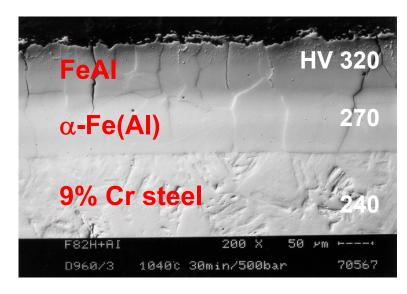
Heat treatment at 980°C / 0.5 h + 760°C / 1.5 h and an applied pressure of >250 bar (HIPing) reduces porosity and transforms the brittle Fe<sub>2</sub>Al<sub>5</sub>-phase into the more ductile phases FeAI and α-Fe(AI)
