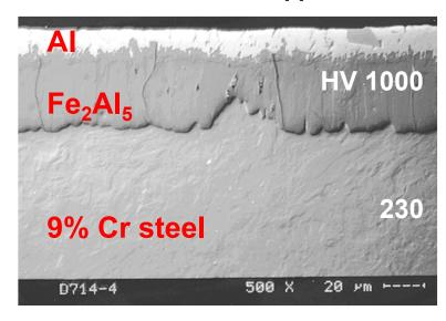
The alloyed surface layer consists of brittle Fe<sub>2</sub>Al<sub>5</sub>, covered by solidified Al
