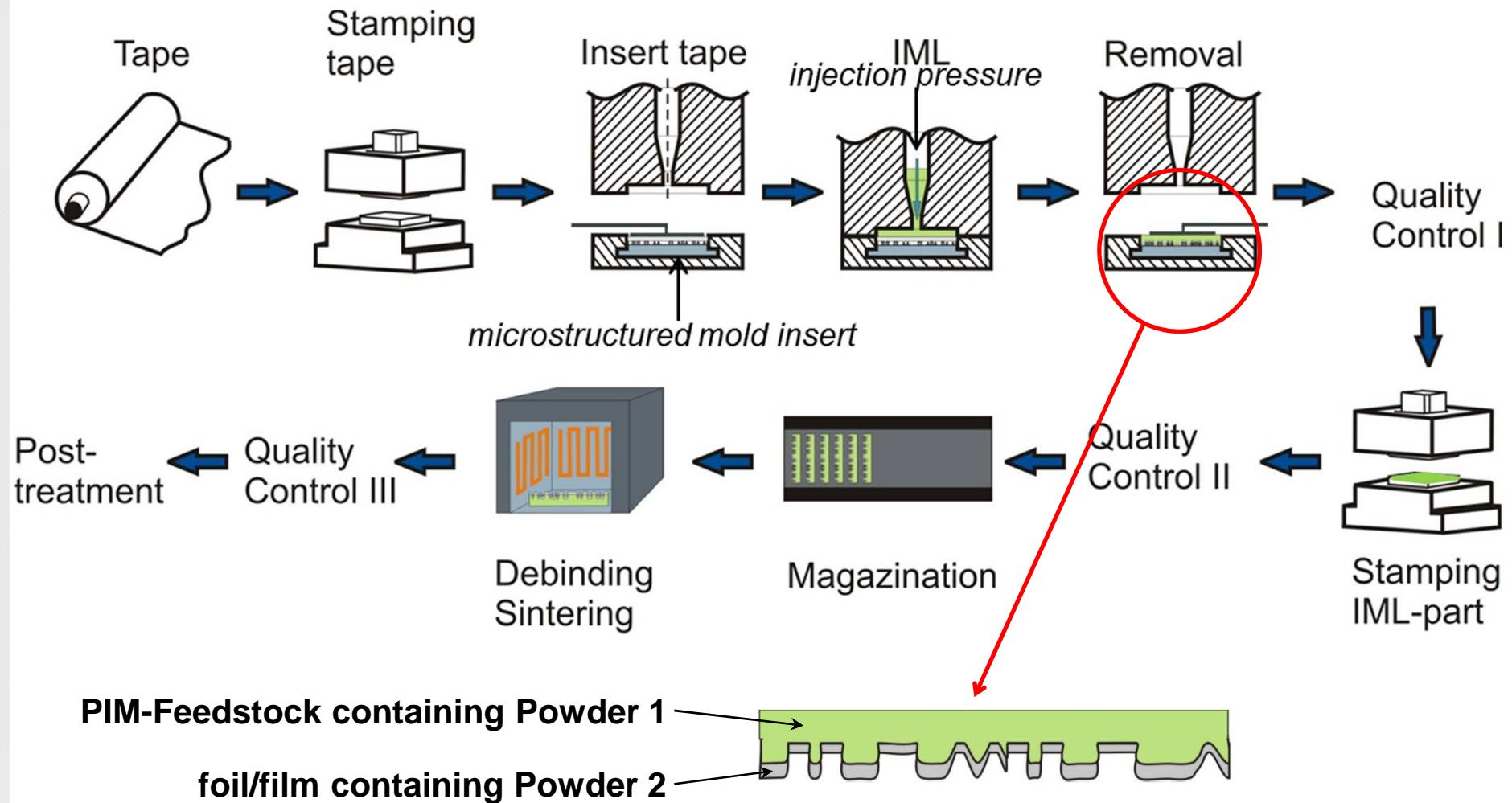
**Powder 2: functional or nano-particles applied on the structured surface**
