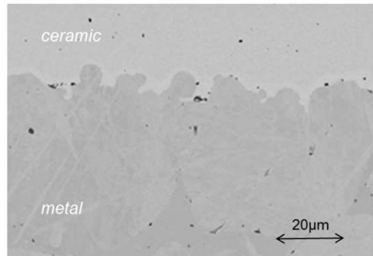
microscopic interlocking structure supported by a partial material bond
