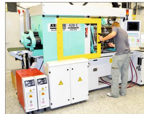
Injection molding of green parts
