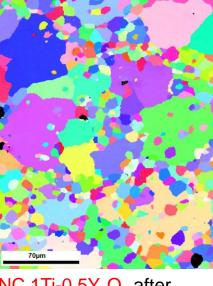
NC 1Ti-0.5Y<sub>2</sub>O<sub>3</sub> after 100 h at 1100 °C
