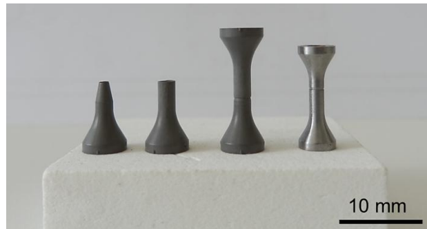
Figure 5: Tensile specimen for sinter joining: green pair of test specimen, green mounted assembly and sinter joined assembly
