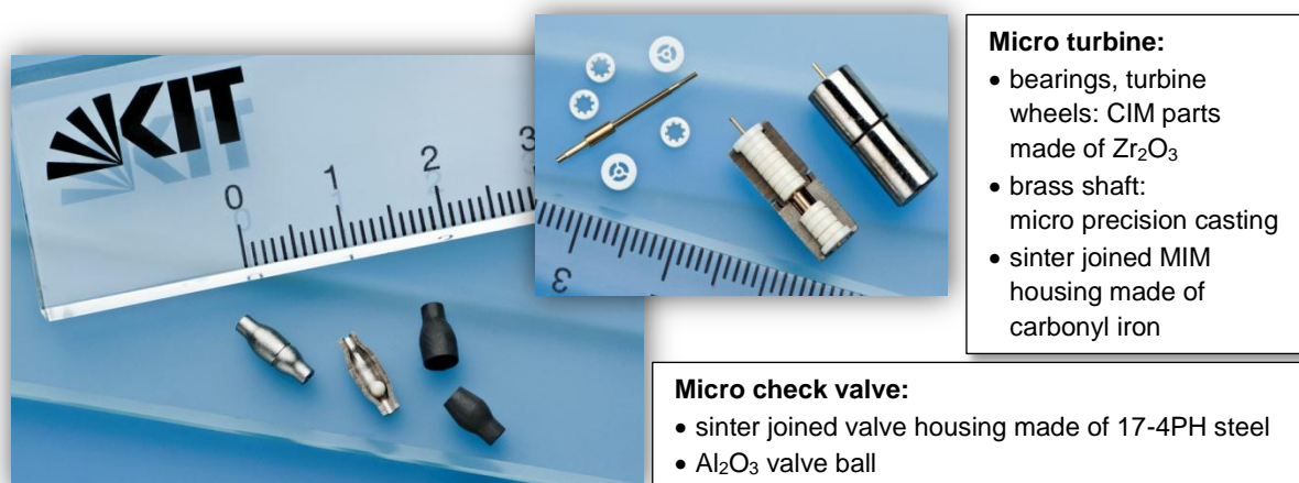
Figure 1: complex \mu -assemblies created with the help of MIM sinter joining: on the left \mu -check valve, on the right: demonstrator of the SFB 499 "micro casting": casted micro turbine
