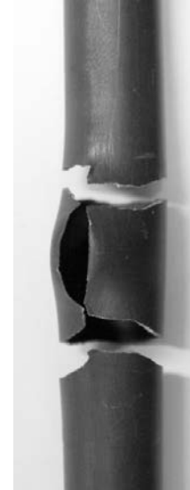
QUENCH-L0 (Zry-4), rod#2: brittle double rupture during tensile tests, fracture stress 400 MPa, elongation 1%; to comparison rupture after necking: fract. elong. 10%
