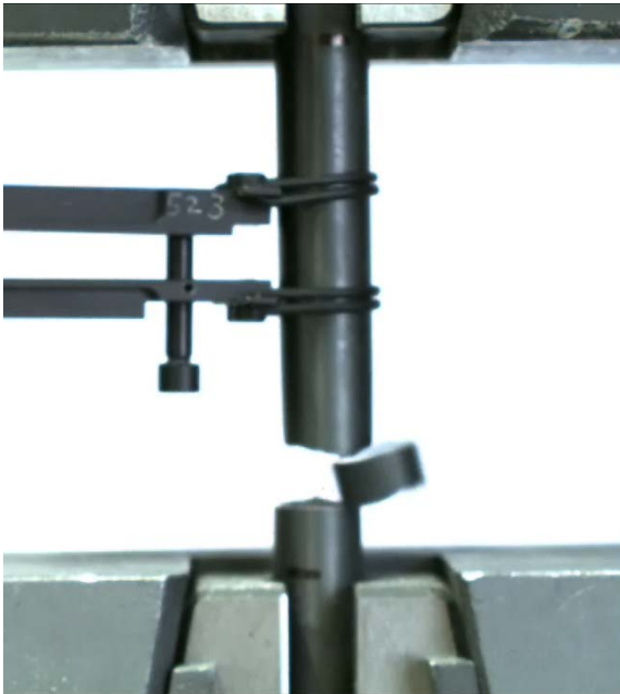
M5 cladding pre-hydrated from outer side to 1700 wppm at 800°C: double rupture during tensile test
